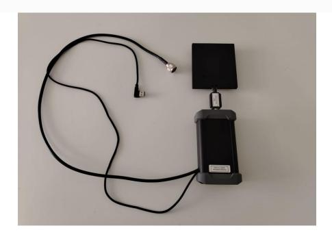
The probe consists of a main unit, a filter, and a directional antenna.
