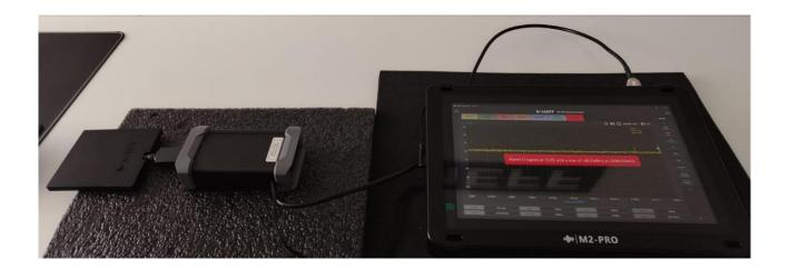
The probe can be used in a **vertical position** when dealing with **very powerful transmission signals** to ensure **effective detection** without risking **receiver saturation**.
